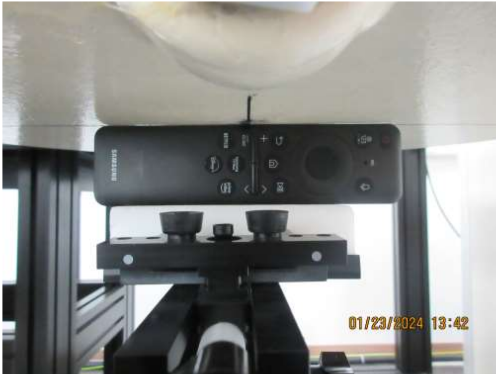
Left from SAM(Flat) Phantom (Separation Distance: 0 cm)
