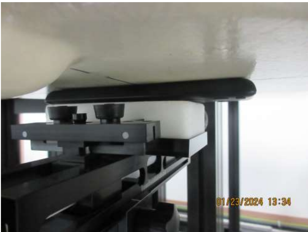
Rear from SAM(Flat) Phantom (Separation Distance: 0 cm)
