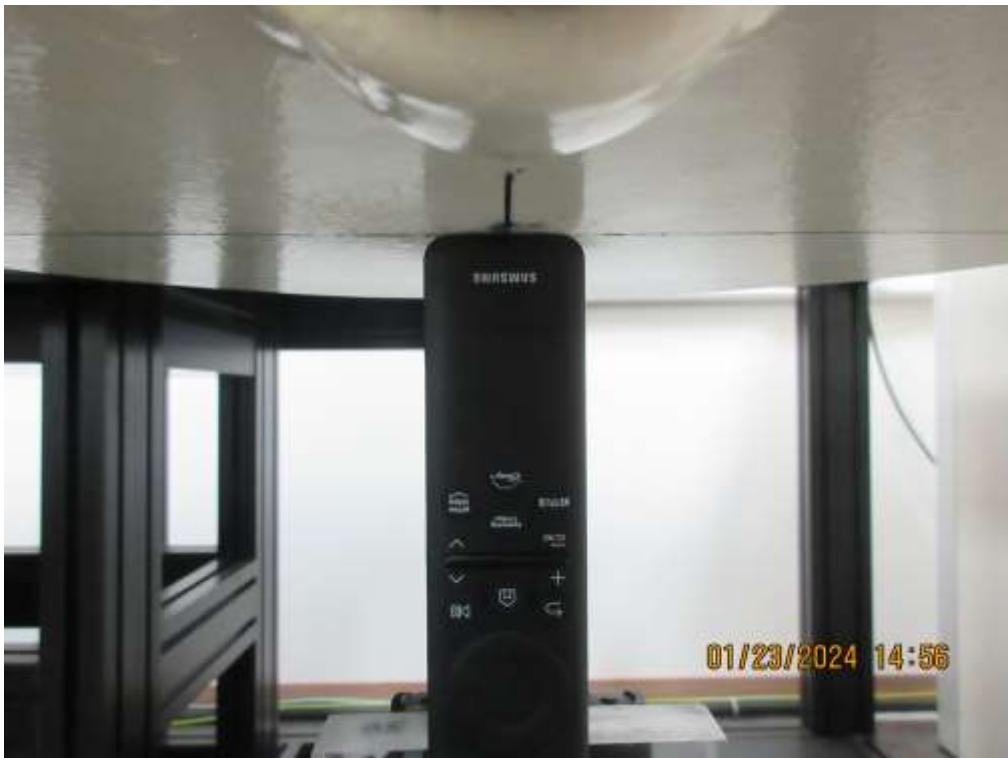
Bottom from SAM(Flat) Phantom (Separation Distance: 0 cm)
