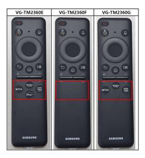
The difference between the models is simply the number of CP (Content Provider) buttons on the exterior of the case. The internal circuitry of the models is exactly the same. The device remain electrically, Software Configuration and mechanically identical to the originally
