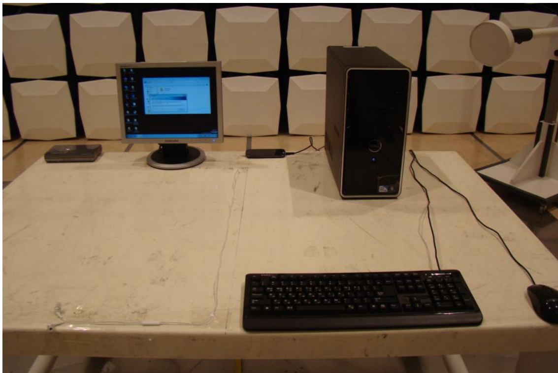
[ Radiated Disturbance for Below 1 GHz – Front ]
