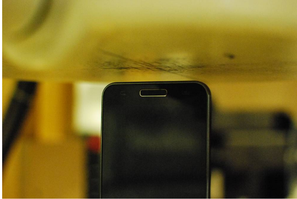
SAR Test Setup Photo 7 – Bottom at 1.0 cm
