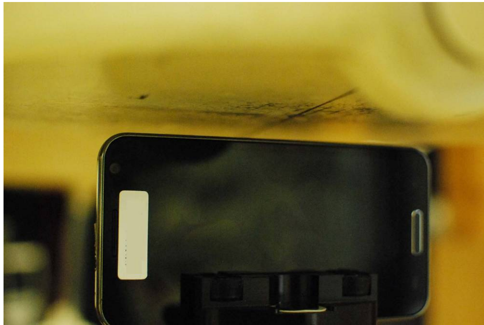
SAR Test Setup Photo 8 – Right at 1.0 cm
