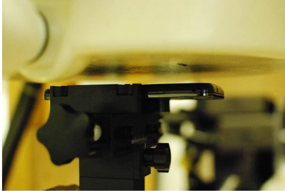
SAR Test Setup Photo 5 – Back at 1.0 cm
