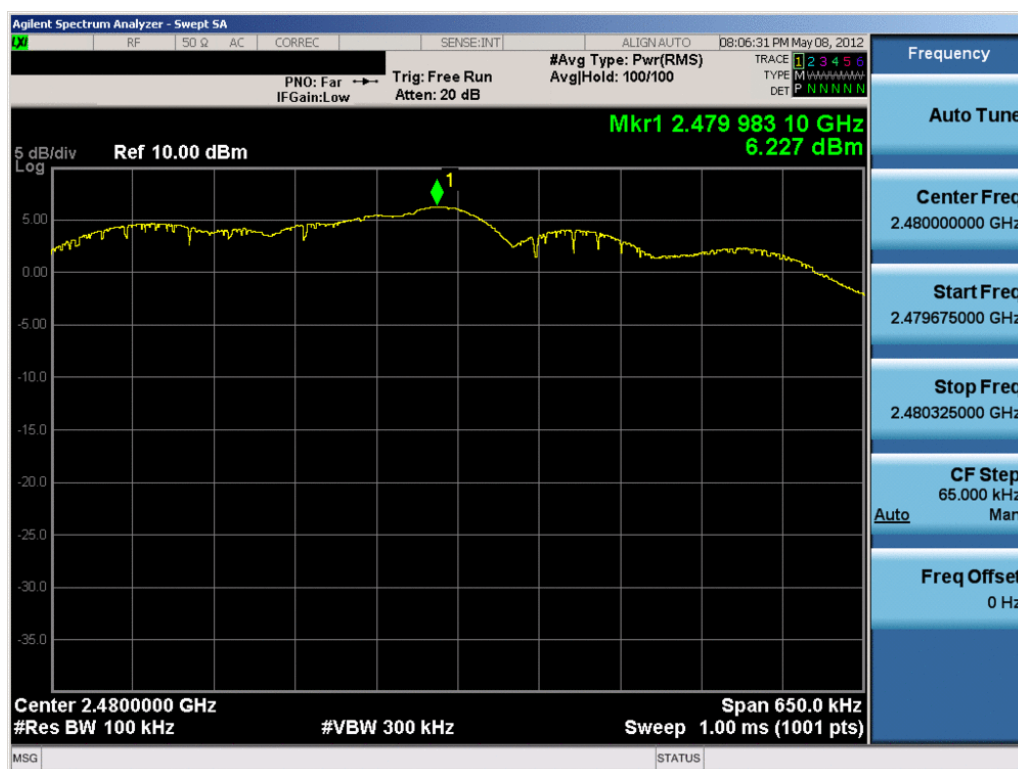
Plot 6-6. Power Spectral Density Plot (Bluetooth (LE) – Ch. 39)
