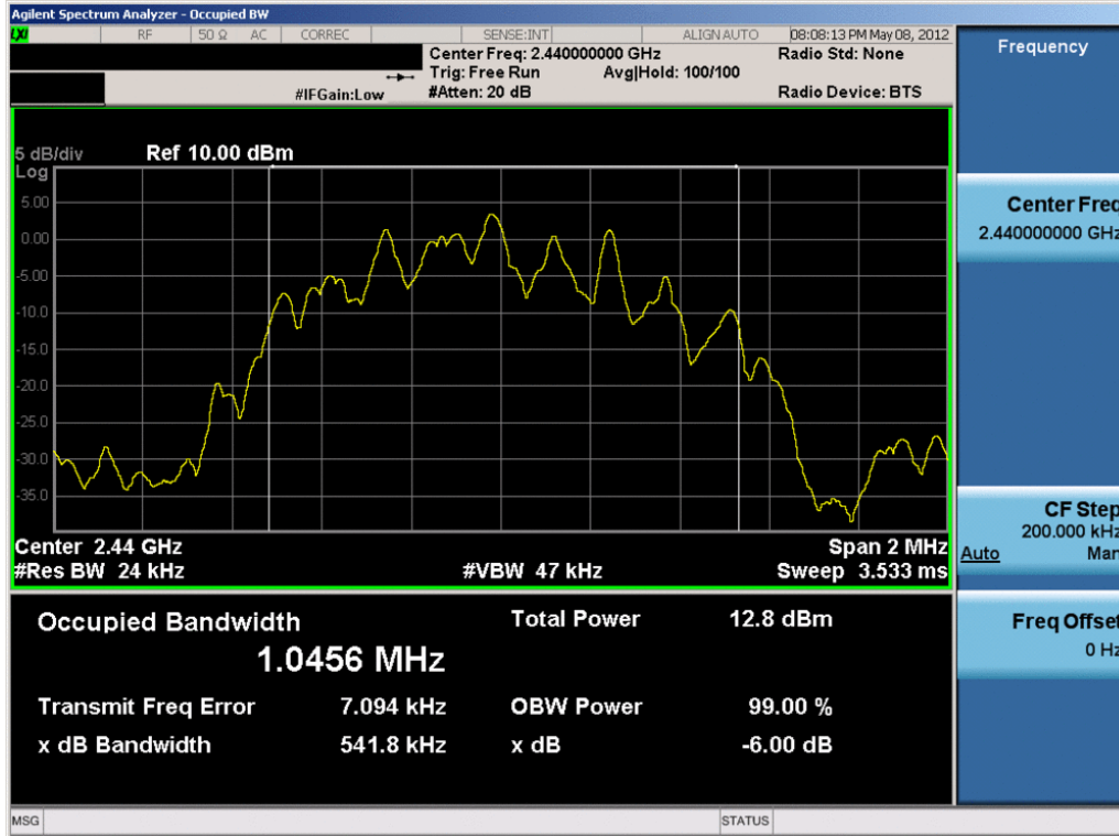
Plot 6-2. 6dB Bandwidth Plot (Bluetooth (LE) – Ch. 19)
