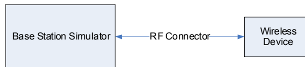
Figure 9-1 Power Measurement Setup
