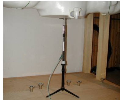
Figure 10-2 System Verification Setup Photo
