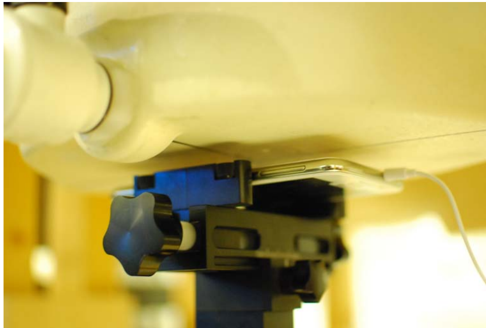
SAR Test Setup Photo 10: Body-Worn at 1.0 cm
