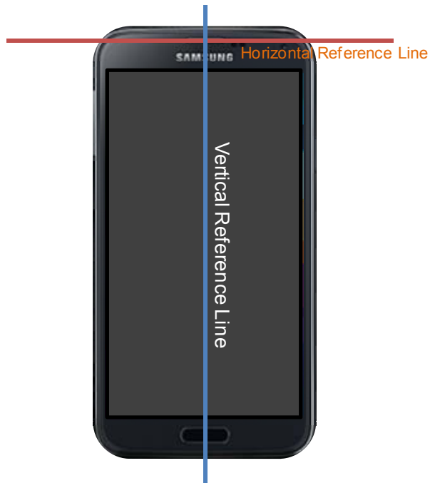
SAR Test Setup Photo 10 – Horizontal and Vertical Reference Lines
