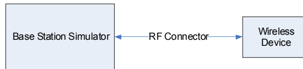
Figure 8-2 Power Measurement Setup
