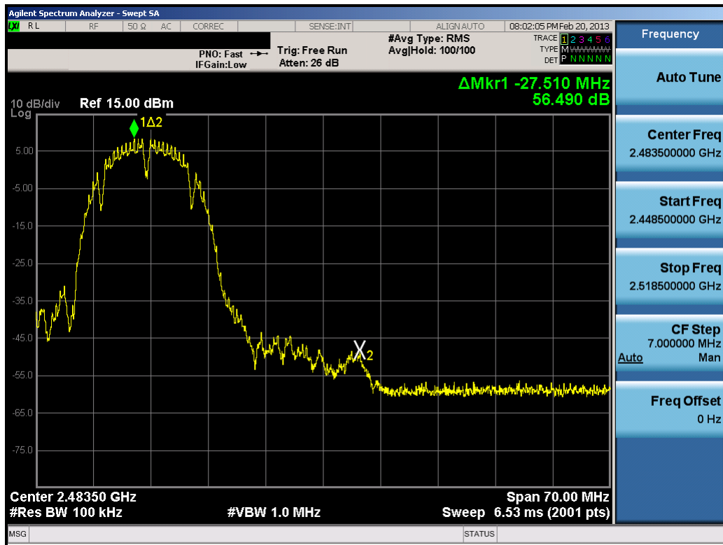
Plot 6-38. Band Edge Plot (802.11b – Ch. 11)
