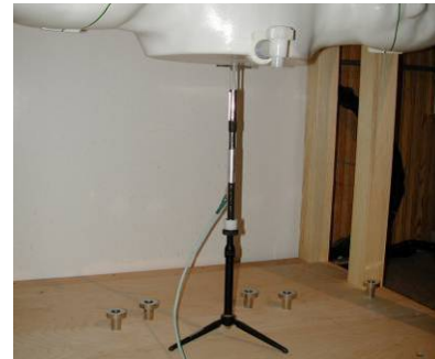
Figure 14-2 System Verification Setup Photo
