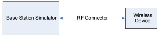
Figure 11-1 Power Measurement Setup
