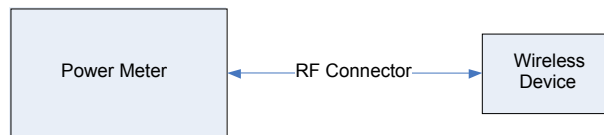
Figure 12-1 Power Measurement Setup
