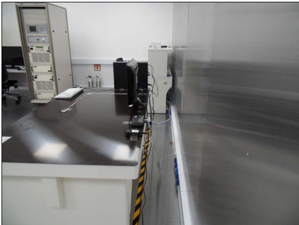
[ Conducted Disturbance – Rear ]
