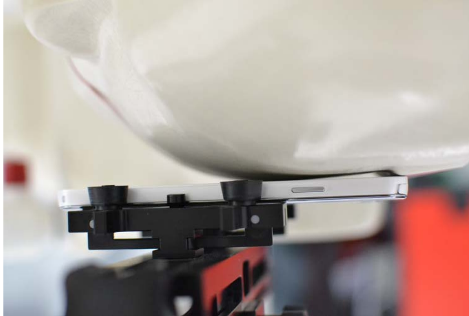
SAR Test Setup Photo 3: Left Cheek
