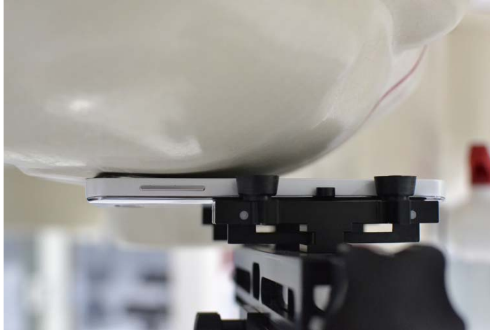
SAR Test Setup Photo 1: Right Cheek
