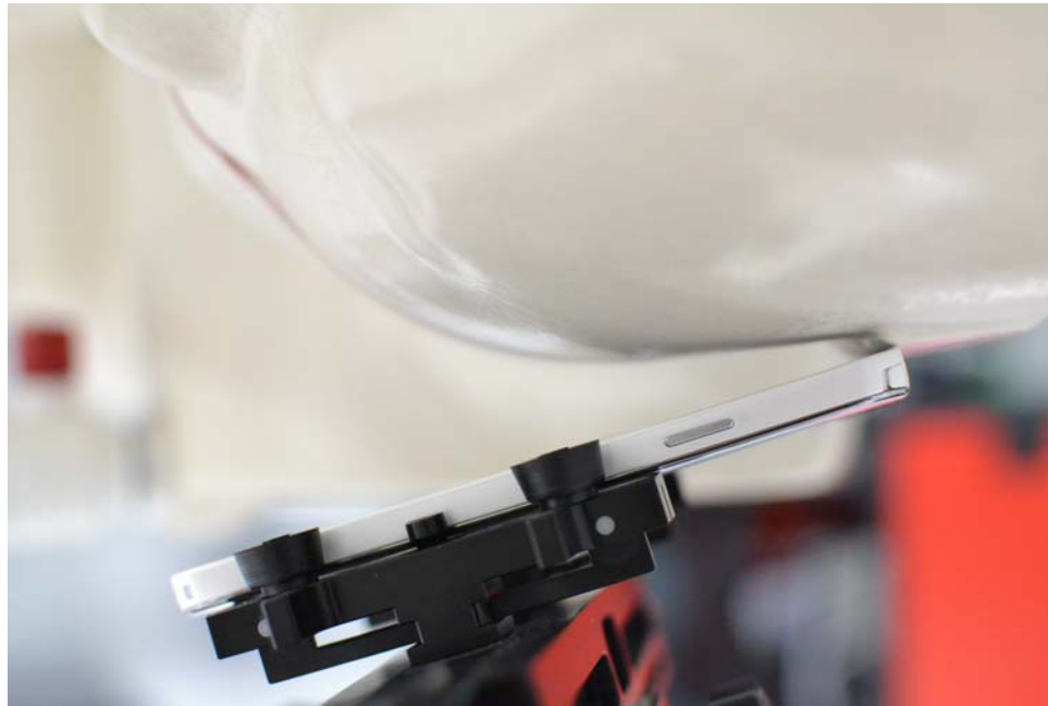
SAR Test Setup Photo 4: Left Tilt
