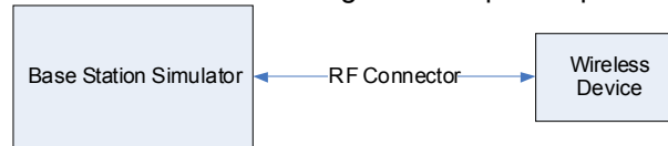
Figure 8-2 Power Measurement Setup
