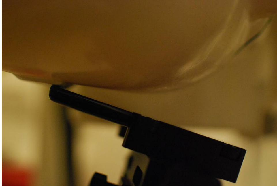
Figure 21-1 SAR Test Setup Photo 1 – Right Touch
