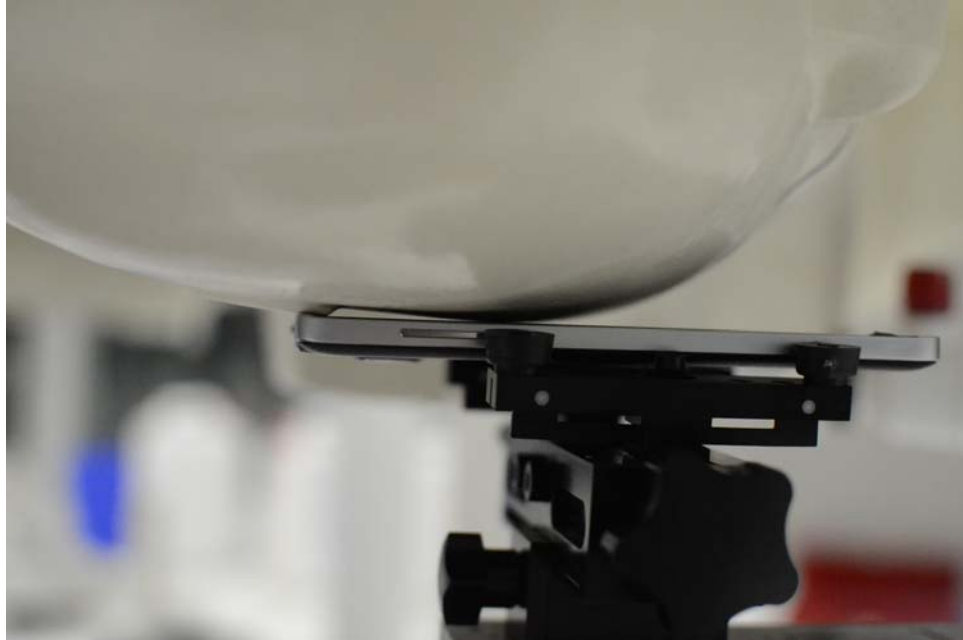
SAR Test Setup Photo 1 – Right Cheek
