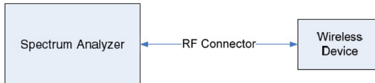
Figure 6-1. Test Instrument & Measurement Setup
