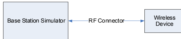
Figure 8-2 Power Measurement Setup
