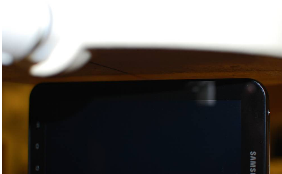
Figure 20-4 SAR Test Setup Photo 4 – Left at 0.5 cm
