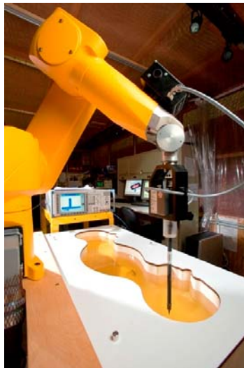
Figure 3-2 DASY4 SAR Measurement System
