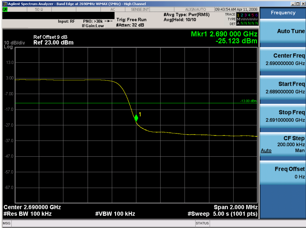
Plot 7-7. Band Edge Plot (WiMAX Mode – High Channel)
