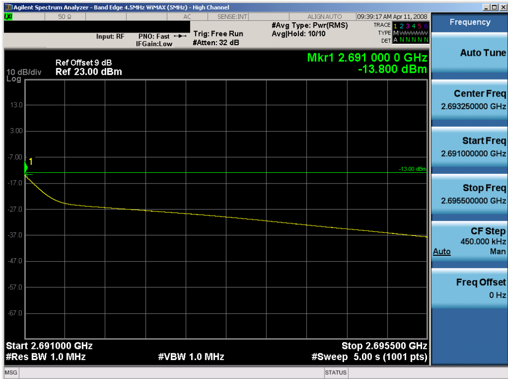
Plot 7-8. 5.5MHz Band Edge Plot (WiMAX Mode – High Channel)
