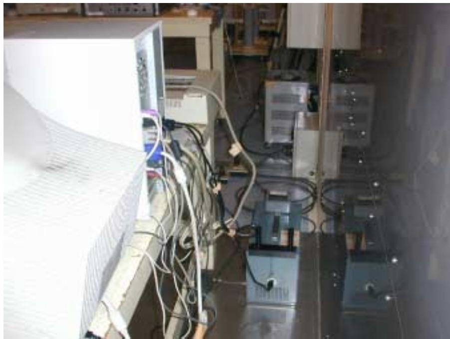
**Photo 7.2** Setup with the Maximized RFI Field Strength Emission Level
