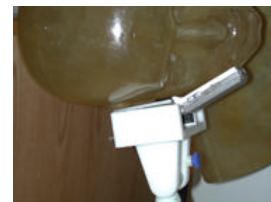
Fig. A Head SAR Test Setup
