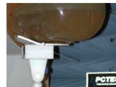
Fig. 14 Head SAR Test Setup
