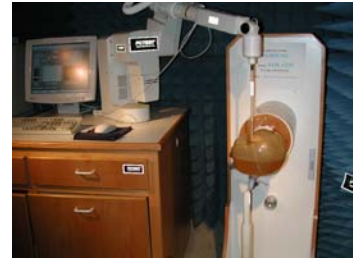
Fig. 1 SAR Test Setup
