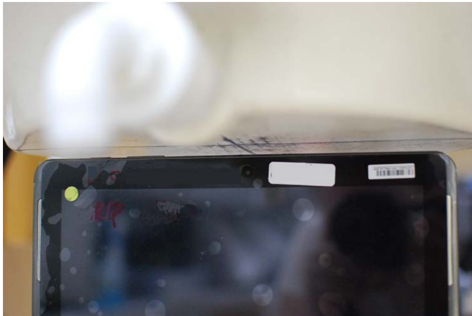
SAR Test Setup Photo 4 – Top Edge at 0.7 cm
