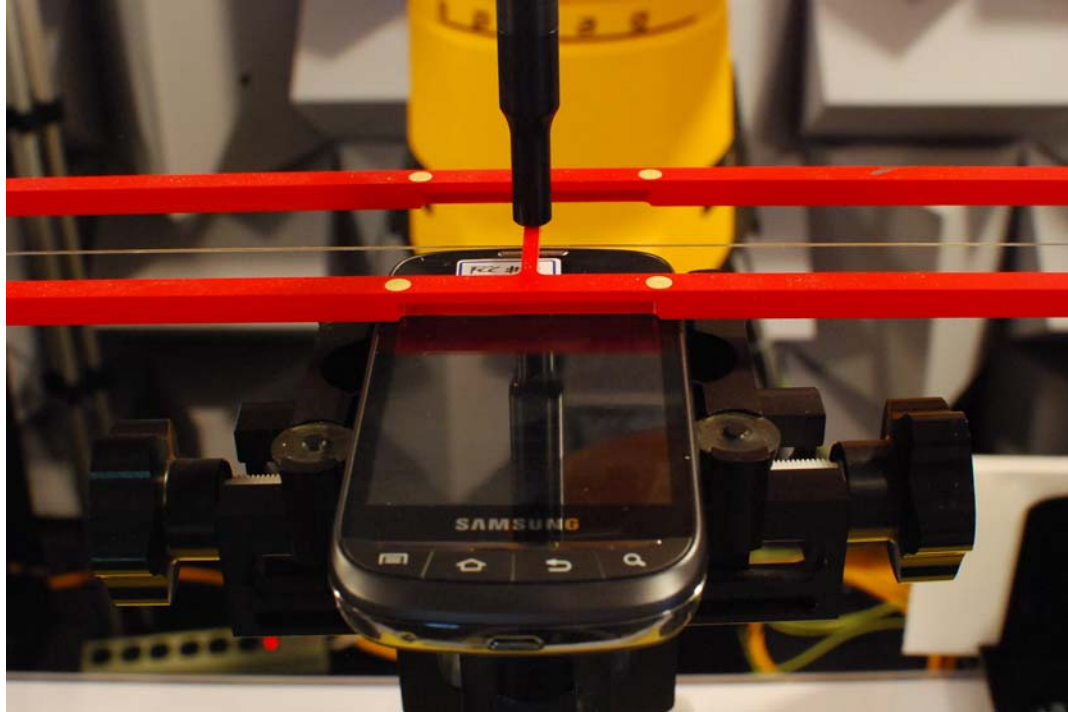
Figure 17-1 Ear Reference Point HAC Phantom Alignment
