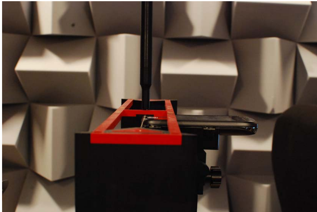
Figure 17-2 HAC Phantom Plane Alignment
