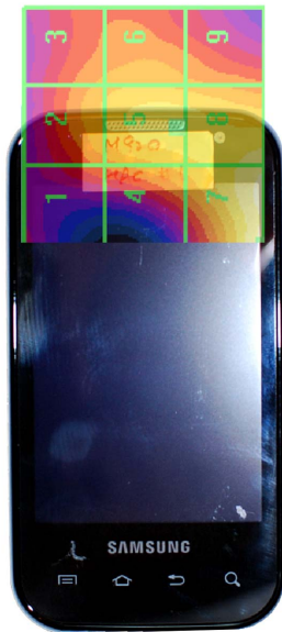
Figure 17-5 H-Field WD Scan overlay
