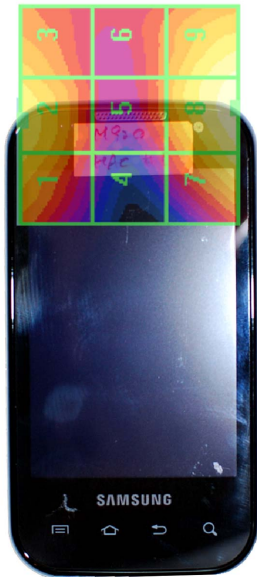
Figure 17-4 E-Field WD Scan overlay
