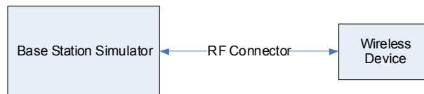
Figure 8-1 Power Measurement Setup
