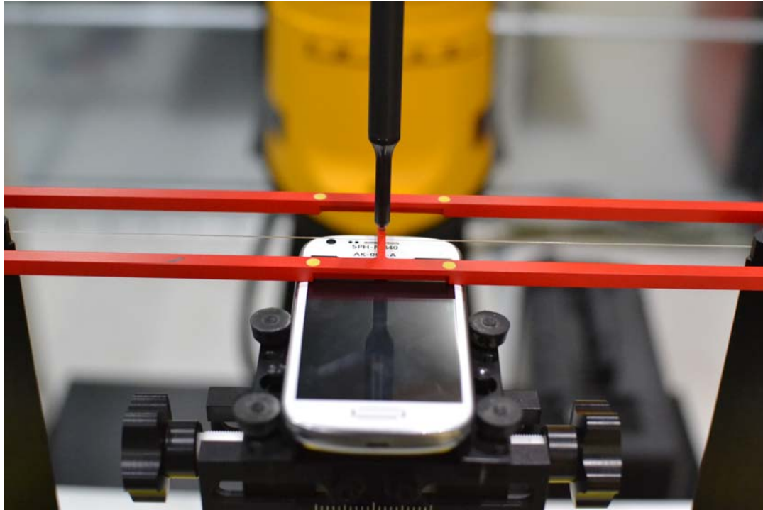
Figure 17-1 Ear Reference Point HAC Phantom Alignment
