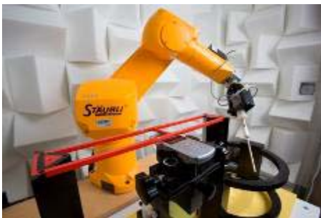
Figure 5-5 SPEAG Robotic System
