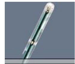
Figure 5-2 H-Field Free-space Probe
