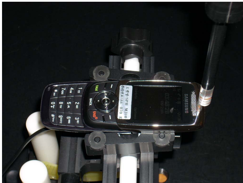
Figure 13-2 Test Setup for Wireless Device
