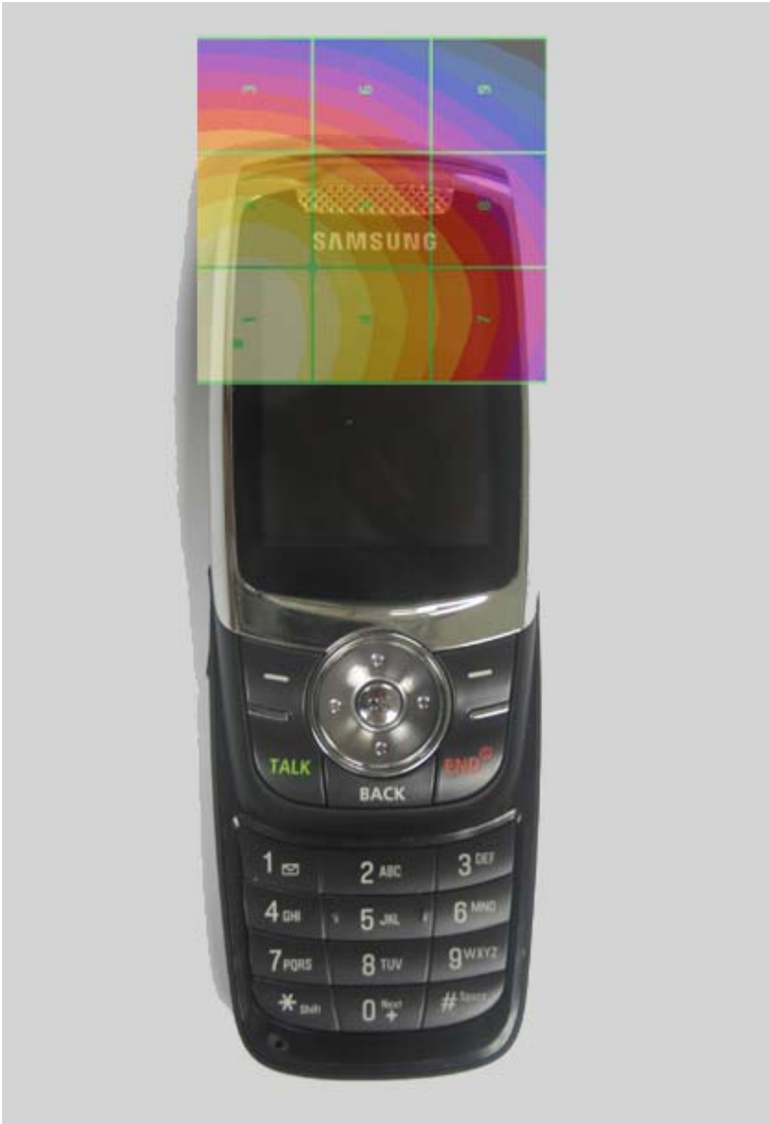
scan overlay with actual device(H-field)-Slide Up
