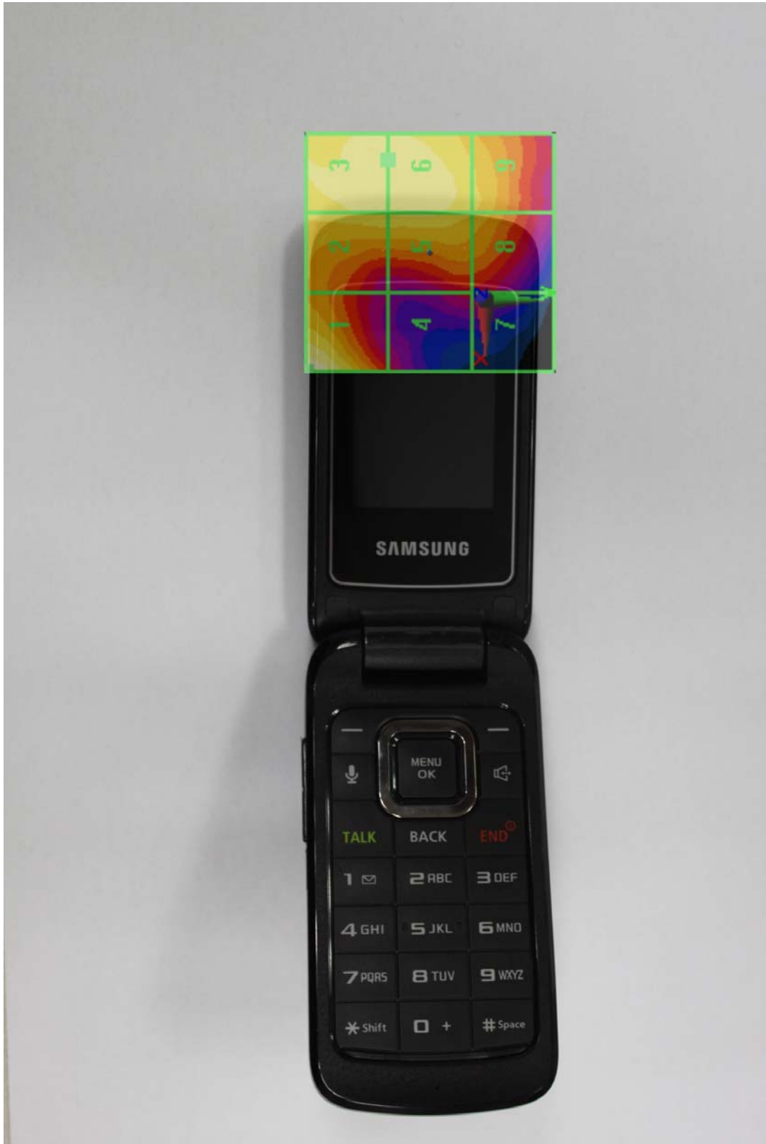
Scan Overlay with actual device(E-Field)
