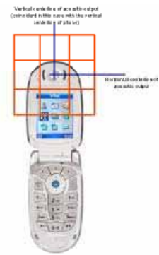
Figure 5.1 Wireless Device and Measurement Plane
