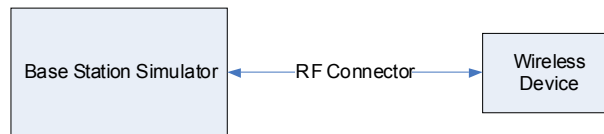
Figure 10-2 Power Measurement Setup
