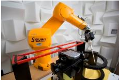
Figure 5-5 SPEAG Robotic System
