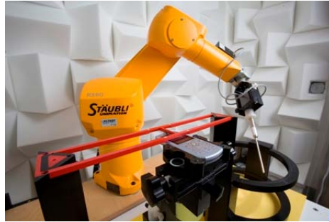
Figure 5-3 SPEAG Robotic System
