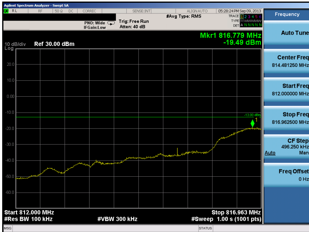
Plot 7-4. Extended Band Edge Plot (Ch. 476)
