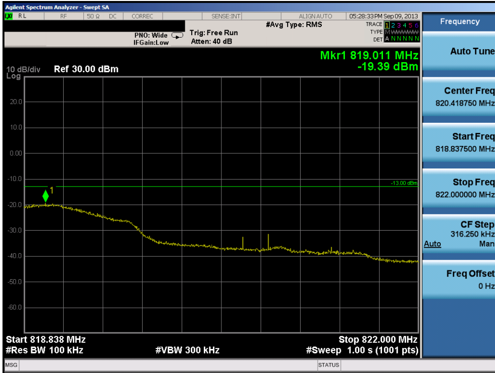
Plot 7-5. Extended Band Edge Plot - Interior (Ch. 476)
