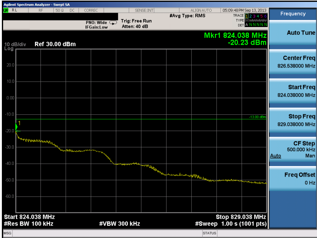
Plot 7-23. Extended Band Edge Plot (1.4MHz QPSK – RB Size 6 – High Channel)
