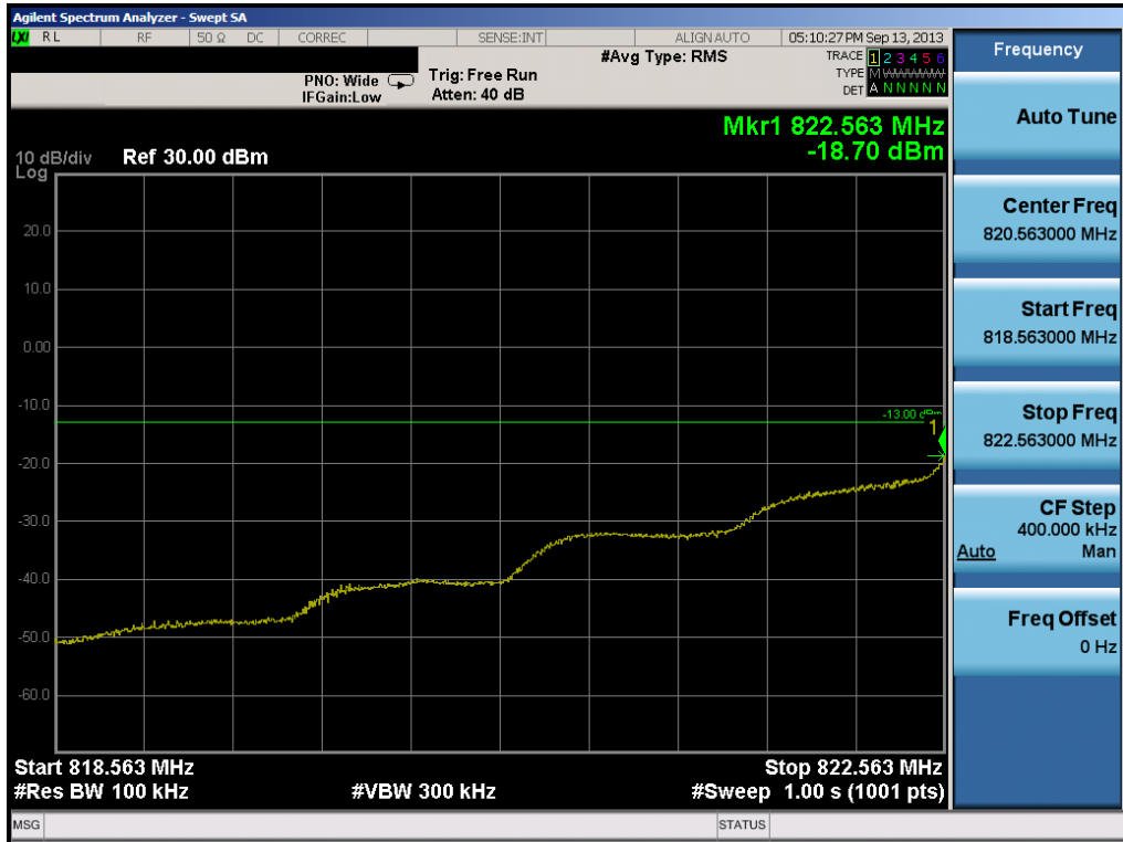
Plot 7-24. Extended Band Edge Plot (1.4MHz QPSK – RB Size 6 – High Channel)
