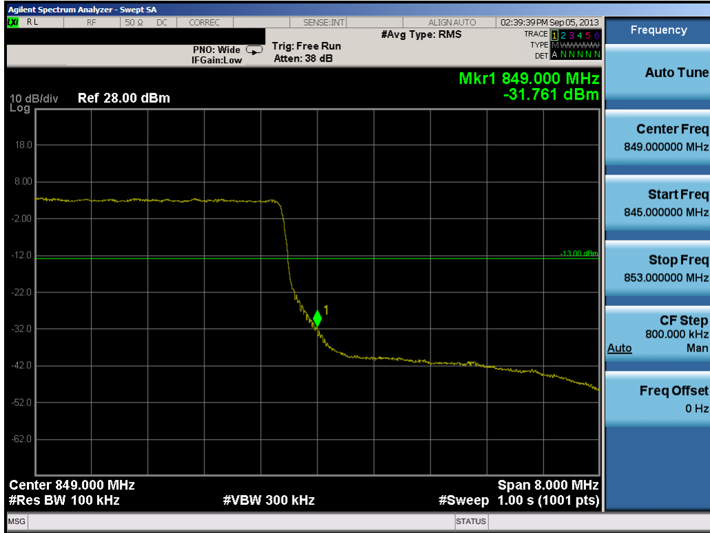
Plot 7-22. Upper Band Edge Plot (10.0MHz QPSK – RB Size 50)
