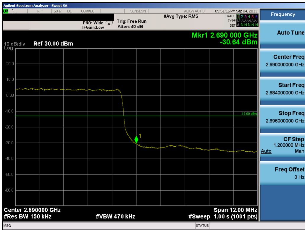
Plot 9-19. Upper Band Edge Plot (15.0MHz QPSK – RB Size 75)
