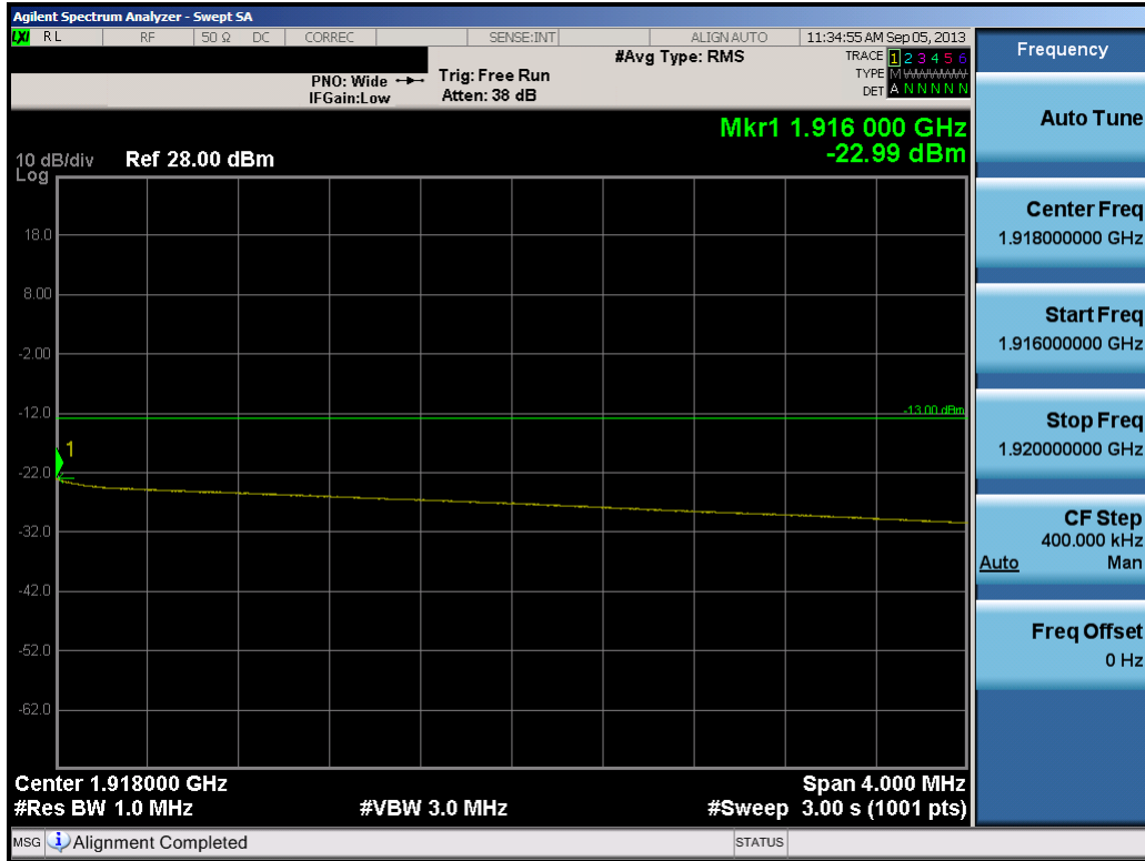
Plot 8-28. Upper Extended Band Edge Plot (10.0MHz QPSK – RB Size 50)
