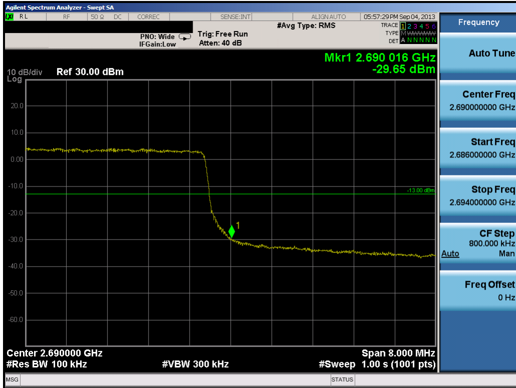
Plot 9-4. Upper Band Edge Plot (10.0MHz QPSK – RB Size 50)
