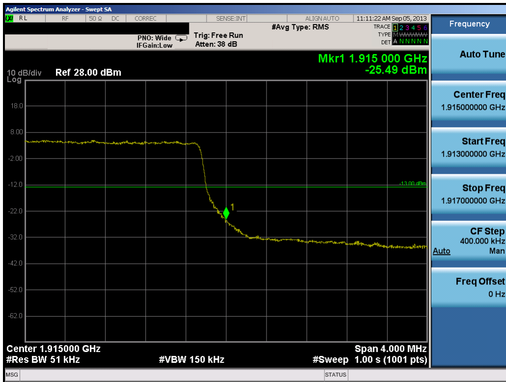
Plot 8-19. Upper Band Edge Plot (5.0MHz QPSK – RB Size 25)
