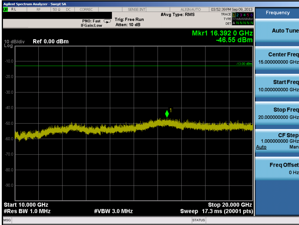
Plot 6-47. Conducted Spurious Plot (PCS WCDMA Mode – Ch. 9538)
