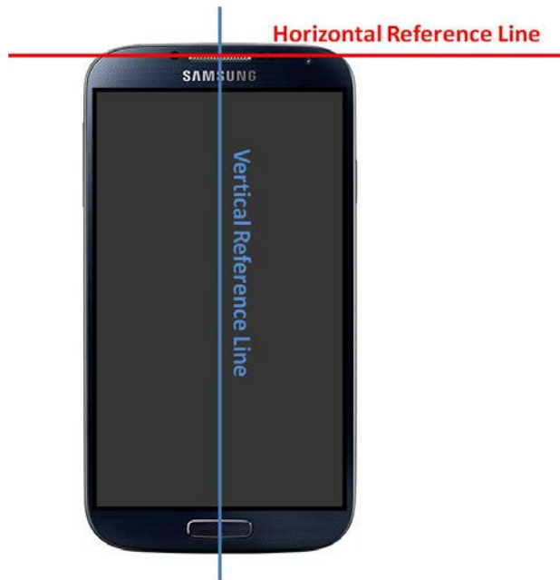
SAR Test Setup Photo 9: DUT Reference Lines
