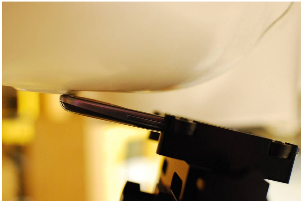
SAR Test Setup Photo 2: Right Tilt
