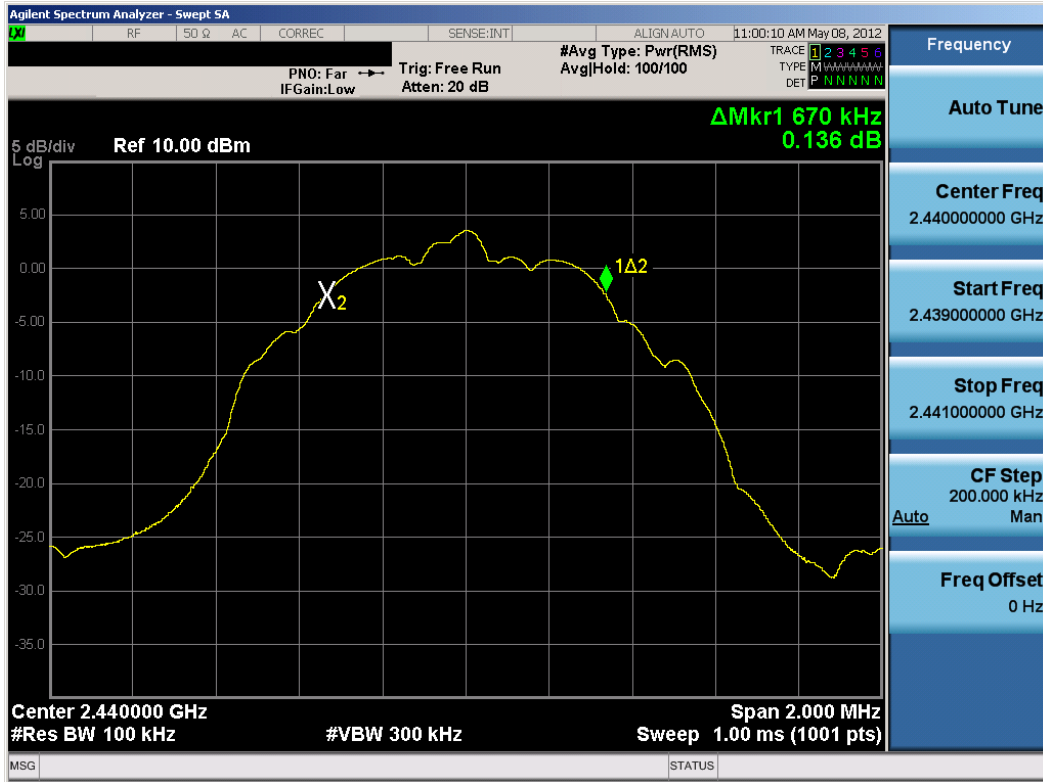
Plot 6-2. 6dB Bandwidth Plot (Bluetooth (LE) – Ch. 19)
