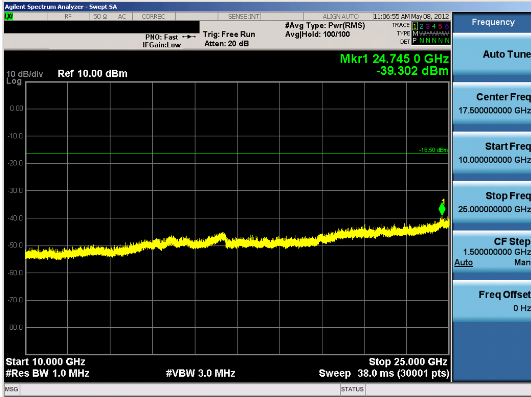
Plot 6-12. Conducted Spurious Plot (Bluetooth (LE) – Ch. 19)
