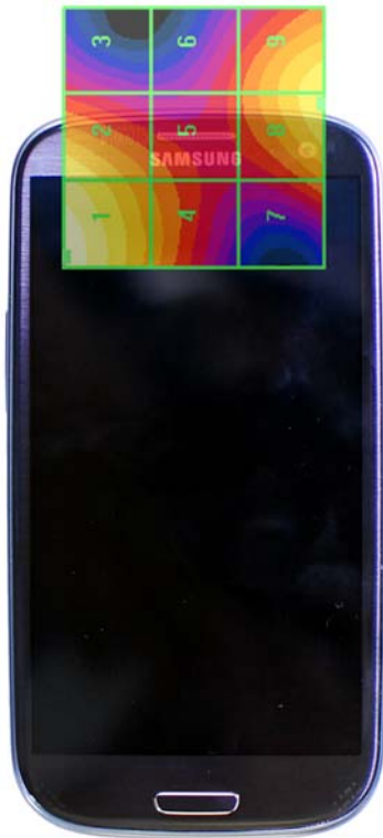
Figure 17-4 E-Field WD Scan overlay
