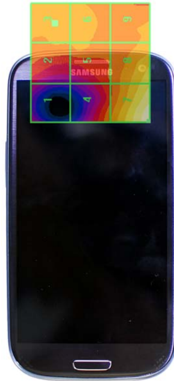
Figure 17-5 H-Field WD Scan overlay
