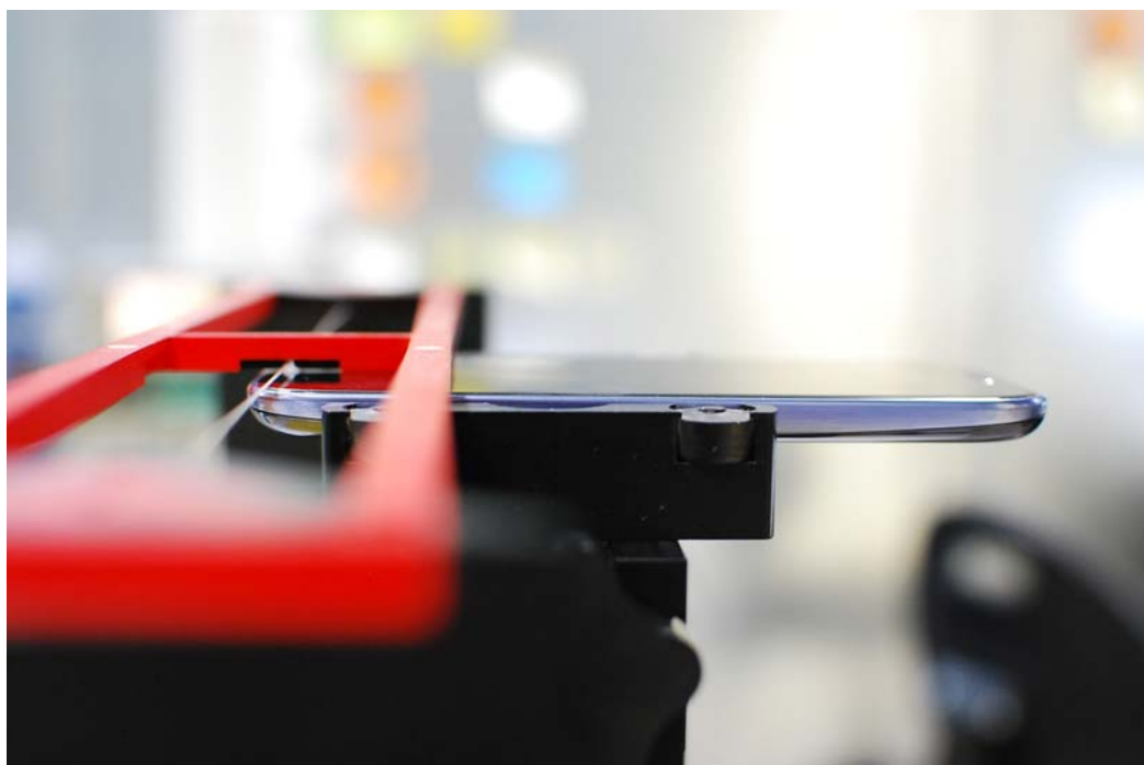
Figure 17-2 HAC Phantom Plane Alignment
