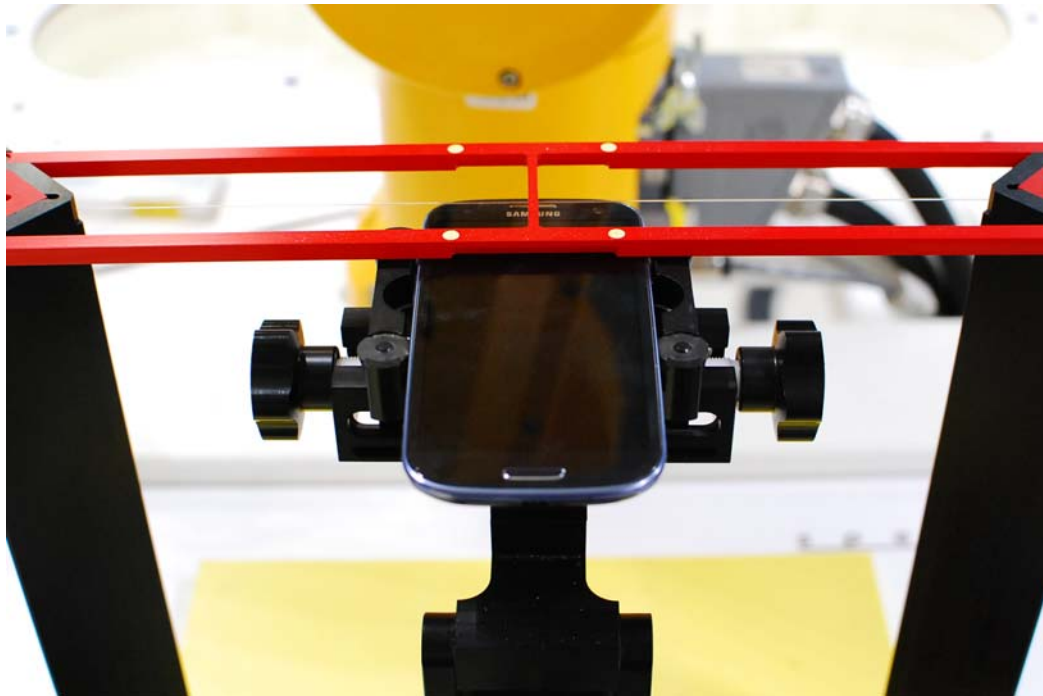
Figure 17-1 Ear Reference Point HAC Phantom Alignment
