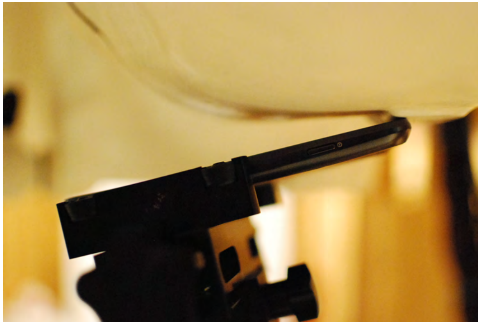
SAR Test Setup Photo 4: Left Tilt
