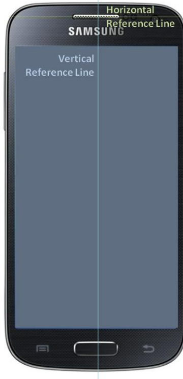
SAR Test Setup Photo 9: Vertical and Horizontal Reference Lines
