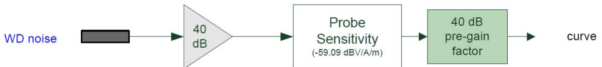
Figure 6-2 Audio Band Magnetic Curve Measurement Block Diagram
