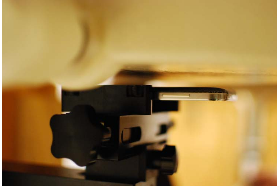
SAR Test Setup Photo 5: Back at 1.0 cm
