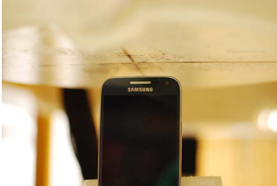
SAR Test Setup Photo 7: Top at 1.0 cm
