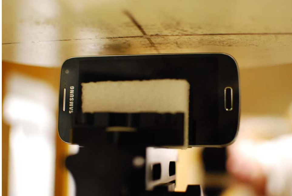
SAR Test Setup Photo 9: Right at 1.0 cm
