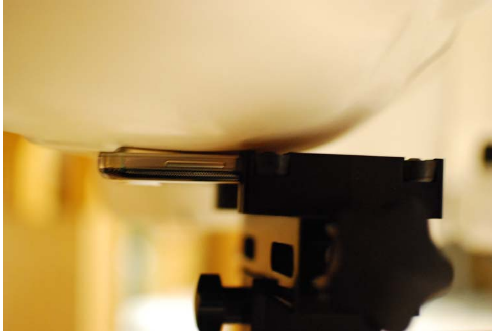
SAR Test Setup Photo 1: Right Cheek
