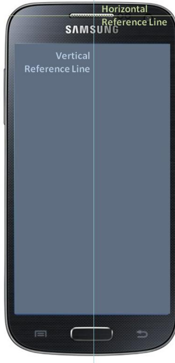
SAR Test Setup Photo 11: Vertical and Horizontal Reference Lines
