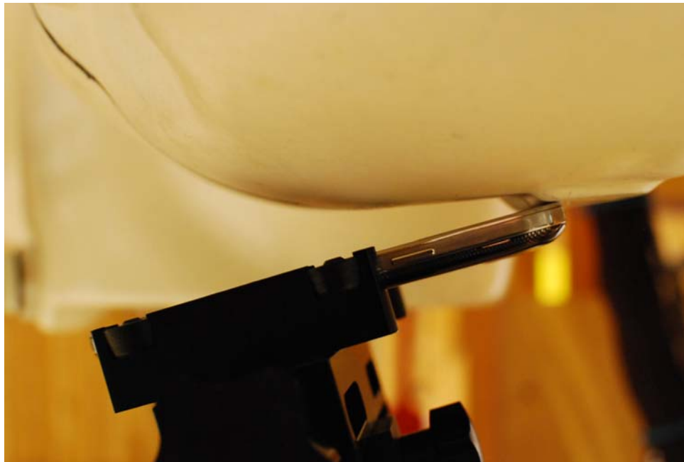
SAR Test Setup Photo 4: Left Tilt
