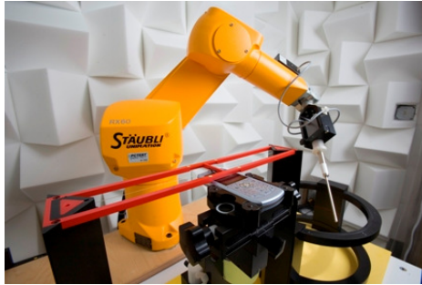
Figure 5-3 SPEAG Robotic System
