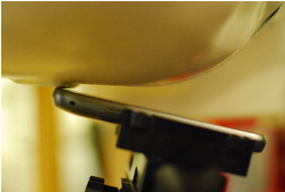
SAR Test Setup Photo 2 – Right Tilt
