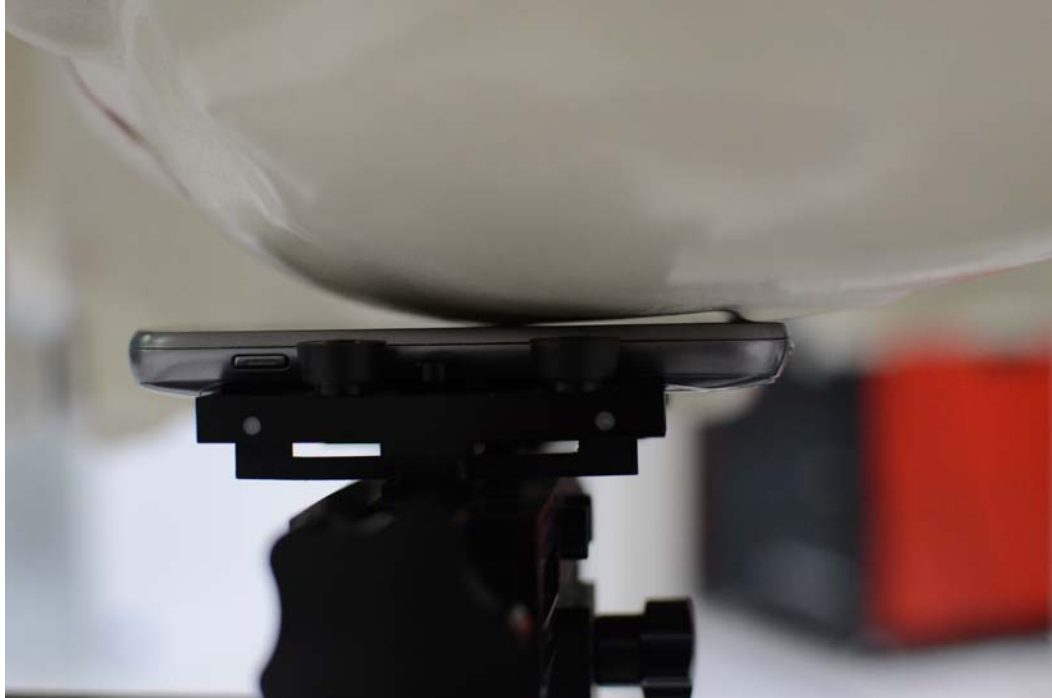
SAR Test Setup Photo 3 – Left Cheek
