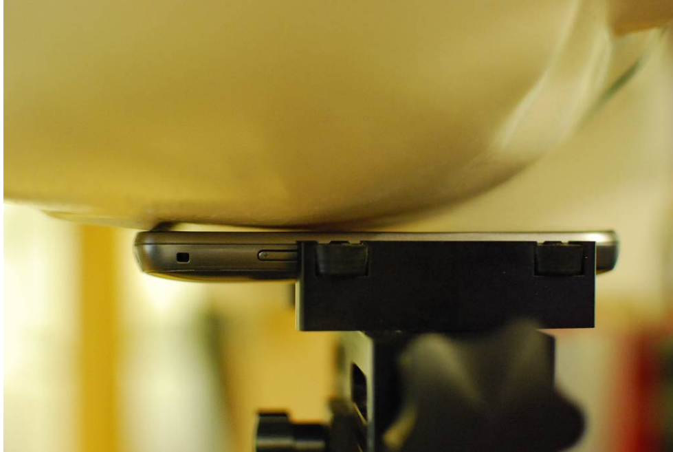
SAR Test Setup Photo 1 – Right Cheek
