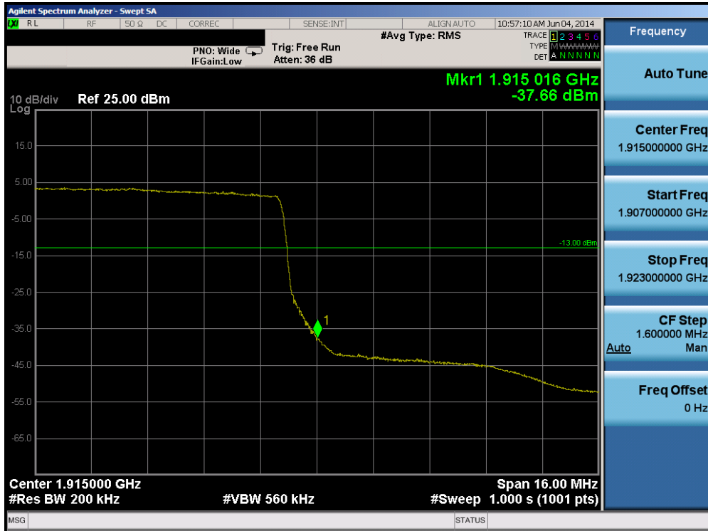
Plot 6-35. Upper Band Edge Plot (Band 25 – 20.0MHz QPSK – RB Size 100)
