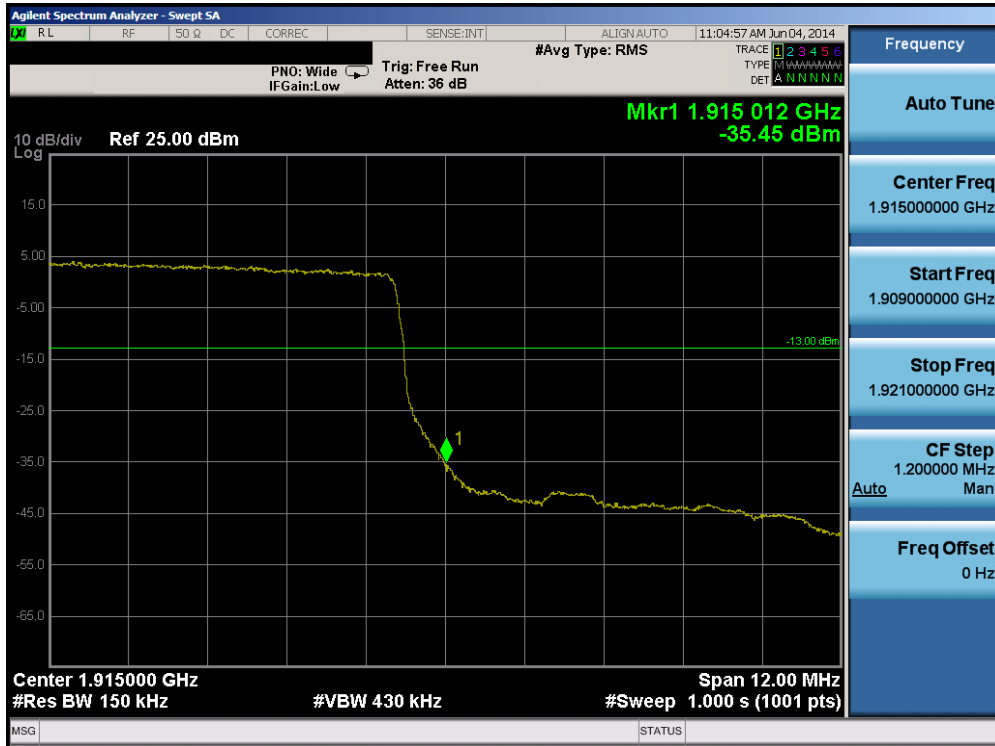
Plot 6-31. Upper Band Edge Plot (Band 25 – 15.0MHz QPSK – RB Size 75)
