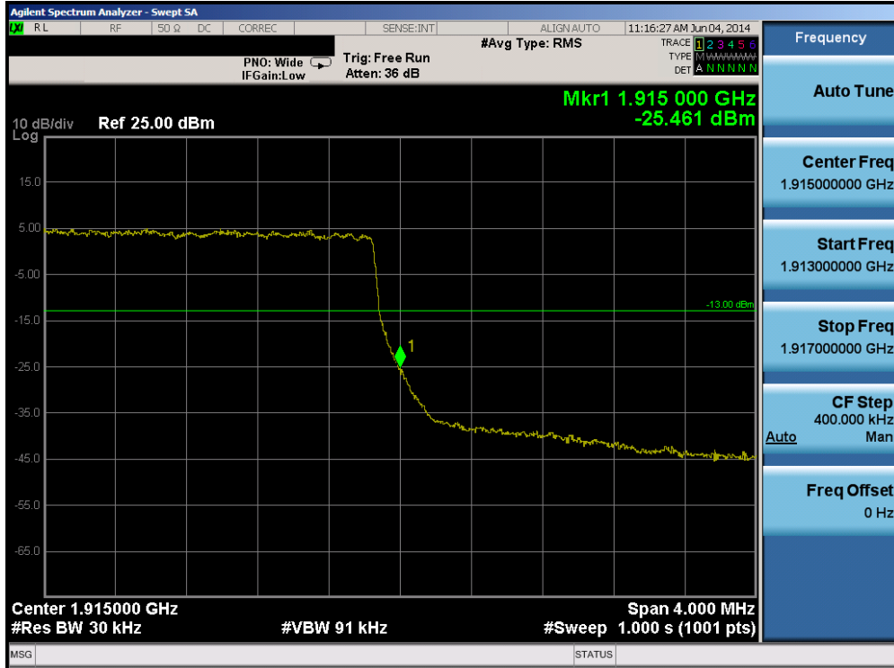
Plot 6-23. Upper Band Edge Plot (Band 25 – 3.0MHz QPSK – RB Size 15)
